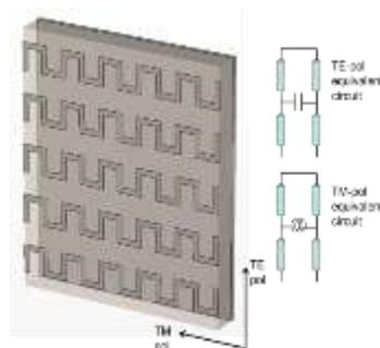
Figure 2. FSS-based absorber
