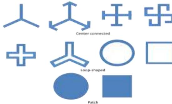
Figure 4. Examples of FSS unit-cells
