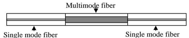
Fig. 1 Schematic diagram of an SMS fiber structure
