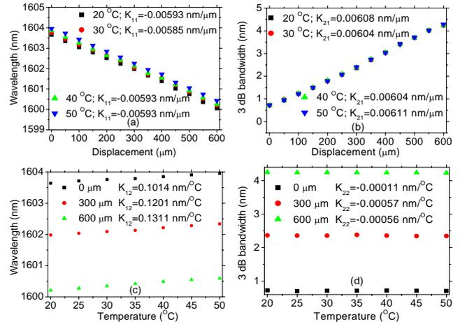
Fig. 5 Measured (a) central wavelength and (b) bandwidth shifts vs. displacement at fixed temperatures and (c) central wavelength and (d) bandwidth shifts vs. temperature at fixed displacements
