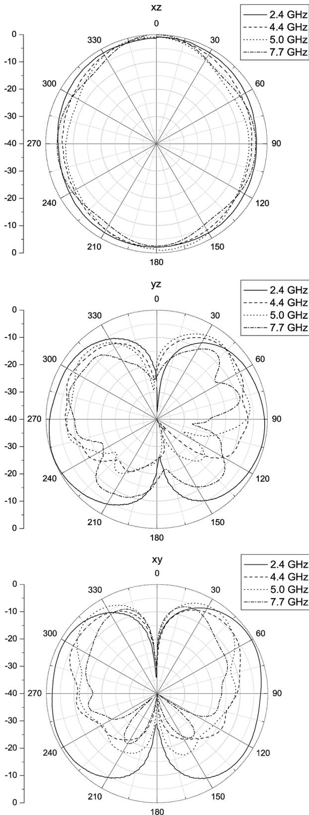
Fig. 4. Measured radiation patterns for the (xz), (yz), and (xy) planes.
