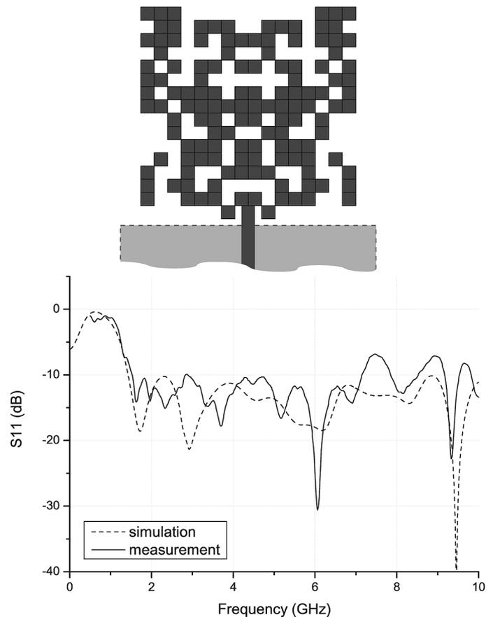
Fig. 3. Antenna geometry optimized for wide bandwidth with simulated and measured return loss.
