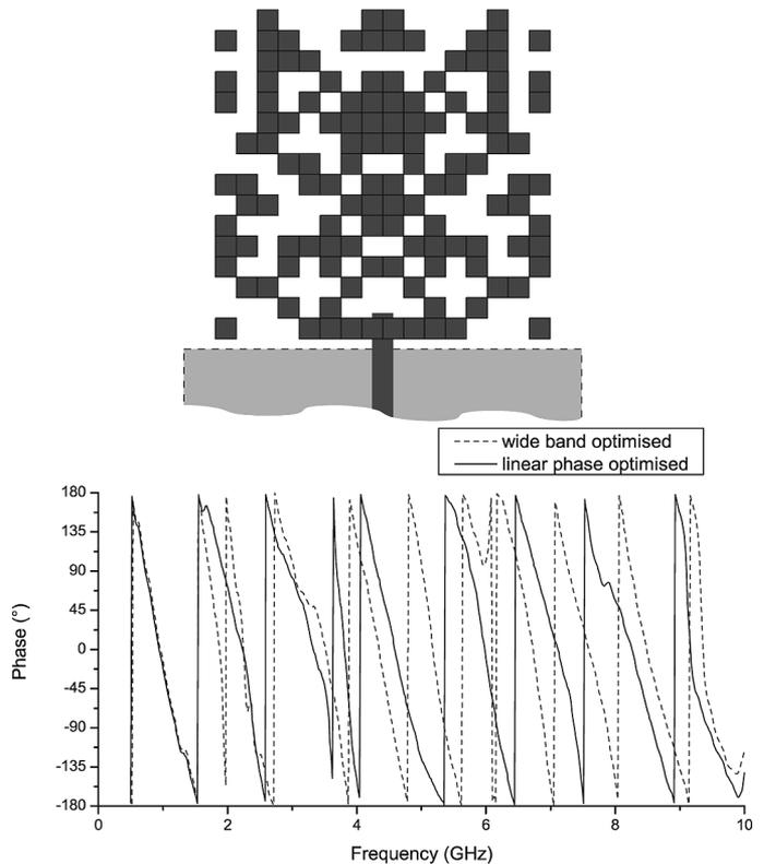
Fig. 5. Antenna geometry optimized for linear phase response with measured phase of the return loss.
