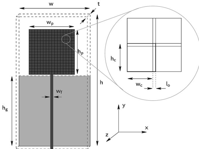
Fig. 2. Antenna geometry and principle of overlapping subpatches.
