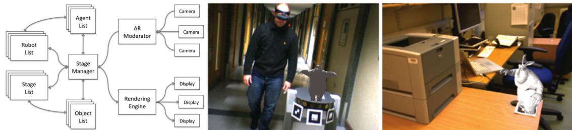
Figure 1: The SOTS architecture; a SOTS agent being followed by a user; and describing a printer.
