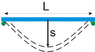
Fig. 3. Scheme of deflection measurements.
