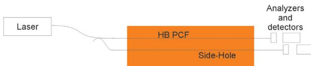
Fig. 1. Schematic of a hybrid sensing system in the intensity domain.
