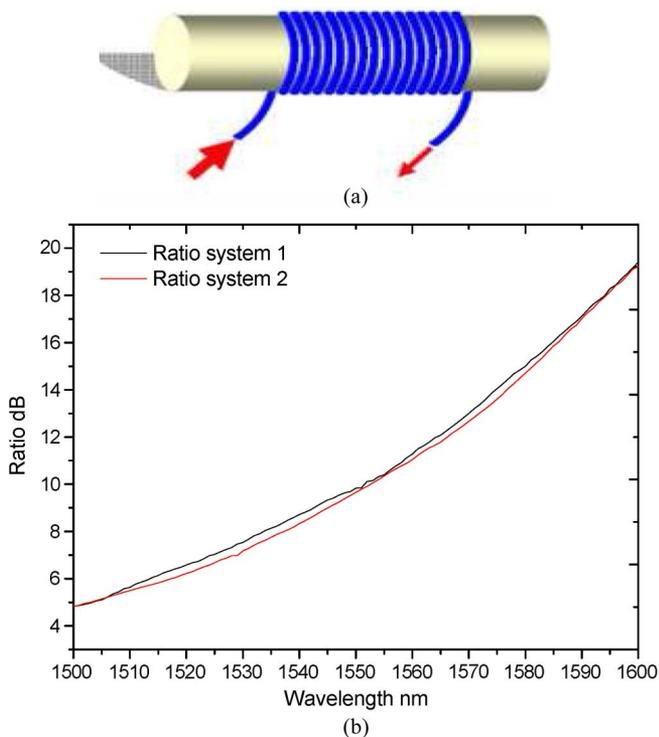
Fig. 6. (a) Schematic of a macrobend fiber filter. (b) Responses of the two fiber filter ratiometric systems.
