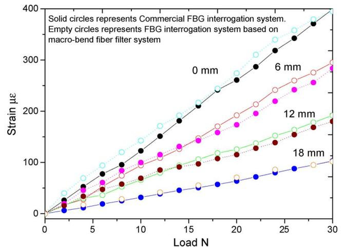
Fig. 12. Comparison of measured strain along the scissor blade at different locations and with different applied loads using a macrobend fiber filter interrogation system and a commercial FBG interrogation system.
