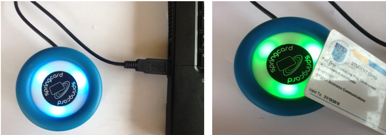
Figure 6.1: Springcard RFID scanner connected via USB port which flashes green on successful student card tag on
