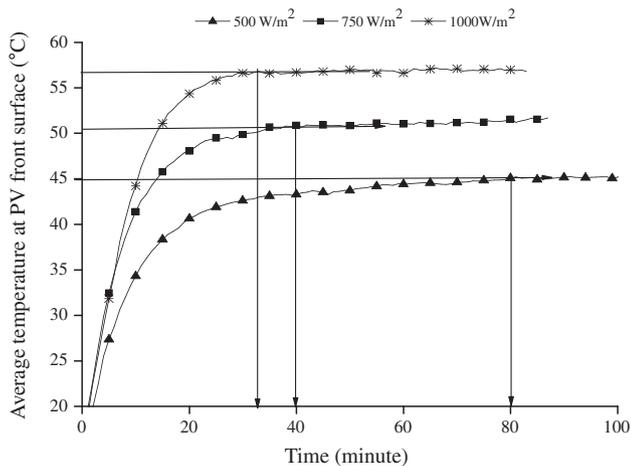
Fig. 4. Reference temperatures at PV front surface at 500 W/m<sup>2</sup>, 750 W/m<sup>2</sup> and 1000 W/m<sup>2</sup> and ambient temperature of 20 ± 1 °C.
