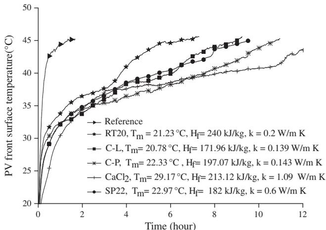
Fig. 5. Temperature evolution on PV front surface in system A at an insolation of 500 W/m<sup>2</sup> and ambient temperature of 20 ± 1 °C.
