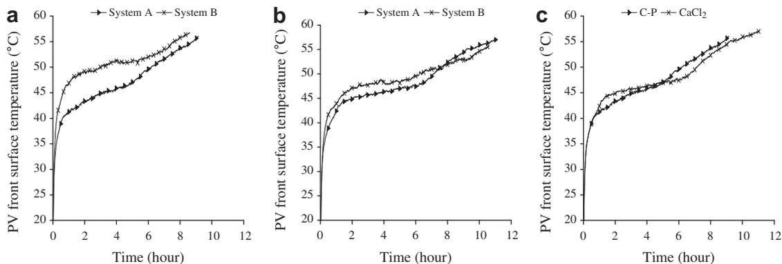
Fig. 11. Temperature at PV front surface using (a) C–P in system A and B (b)  $\text{CaCl}_2$  in system A and B (c) CP and  $\text{CaCl}_2$  in system A at an insolation of  $1000 \text{ W/m}^2$  and ambient temperature of  $20 \pm 1 \text{ }^\circ\text{C}$ .
