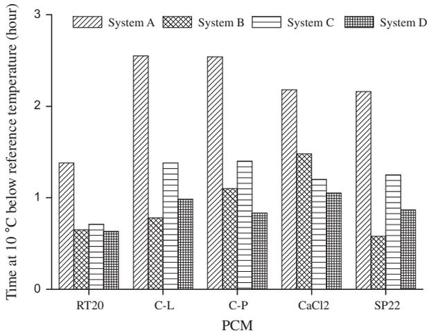
Fig. 6. Duration for which PCM maintained PV front surface temperature 10 °C below the reference temperature in systems A, B, C and D at an insolation of 500 W/m<sup>2</sup> and ambient temperature of 20 ± 1 °C.
