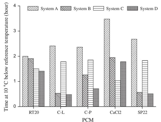
Fig. 8. Duration for which PCM maintained PV front surface temperature 10 °C below the reference temperature in systems A, B, C and D at insolation of 750 W/m<sup>2</sup> and ambient temperature of 20 ± 1 °C.
