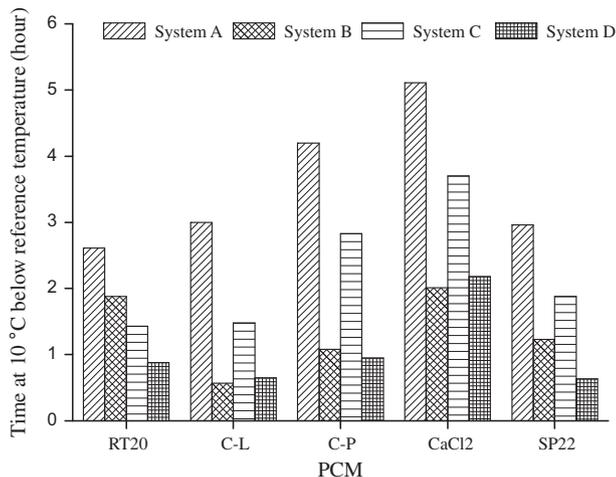
Fig. 10. Duration for which PCM maintained PV front surface temperature  $10 \text{ }^\circ\text{C}$  below the reference temperature in systems A, B, C and D at an insolation of  $1000 \text{ W/m}^2$  and ambient temperature of  $20 \pm 1 \text{ }^\circ\text{C}$ .
