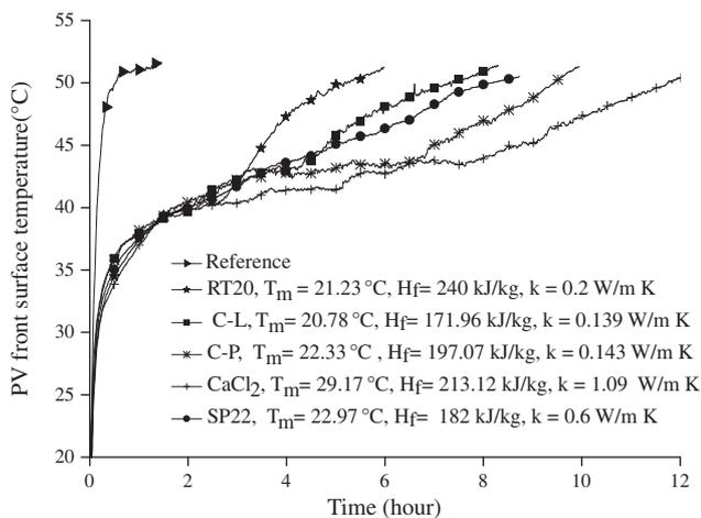
Fig. 7. Temperature evolution on front surface of PV in system A at an insolation of 750 W/m<sup>2</sup> and ambient temperature of 20 ± 1 °C.
