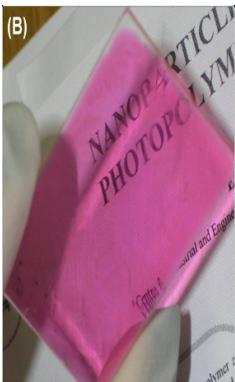
**Figure 3.** (A) SEM of the acrylamide based photopolymer layer (50  $\mu\text{m}$  thickness) doped with Beta nanoparticles (5 wt. %); the scale bar is 50 $\mu\text{m}$  (B) Optically transparent film of acrylamide based photopolymer doped with zeolite A nanoparticles (5 wt. %)
