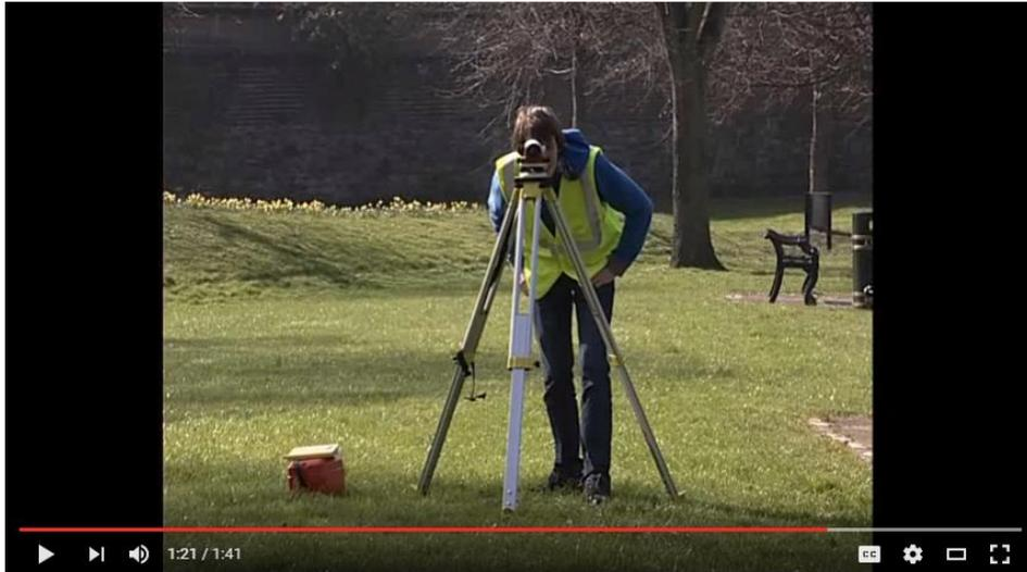
**Figure 1: Levelling with an automatic level**
