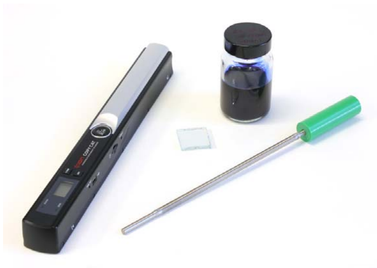
Fig. 1. - The equipment and materials used to conduct the test; a handheld document scanner, the Rz ink, a wire wound rod (K-bar #3) and a sample piece of self-cleaning glass.
