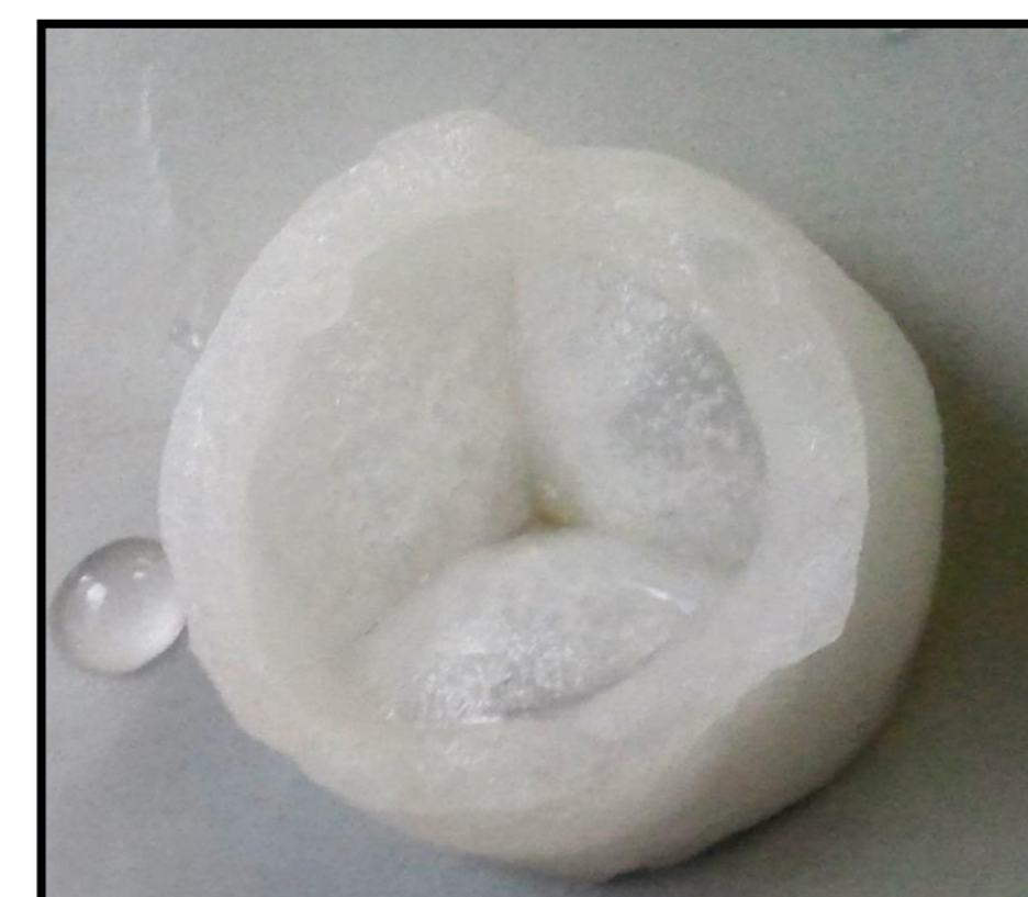
Figure 2. This image shows a sample of the heart valve shaped CG material, post cross-linking and post infiltration with fibrin. The material stands up under its own weight and is easy to handle.
