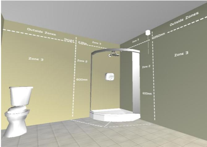
**Figure 4 View of Zones in bathroom in VES**
