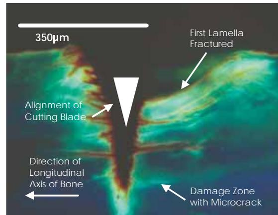
Figure 1: Cutting zone - transverse cutting specimens.
