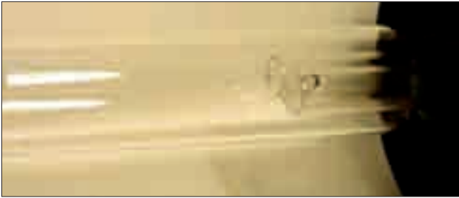
Figure 6: Ultra violet bulb in quartz glass sleeve.
