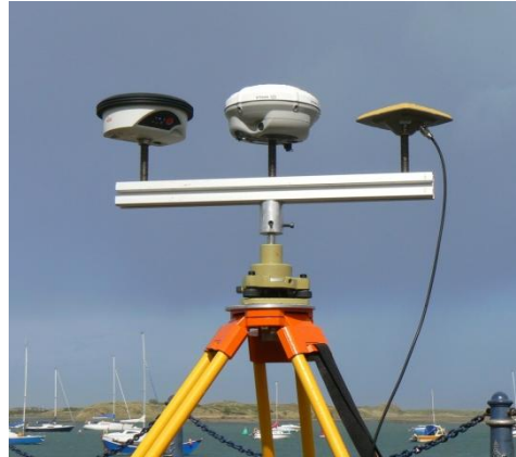
Fig. 5: Bracket allowing simultaneous observation with three receivers.
