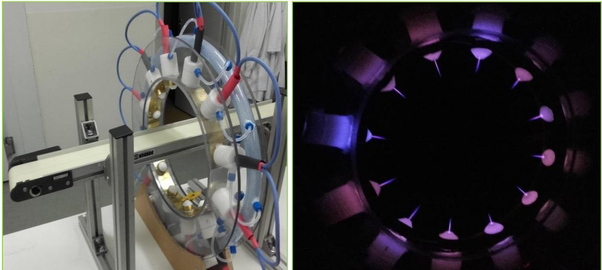
Figure 1. Multi-jet Atmospheric Pressure Plasma discharges designed for food decontamination (DIT BioPlasma Lab)
