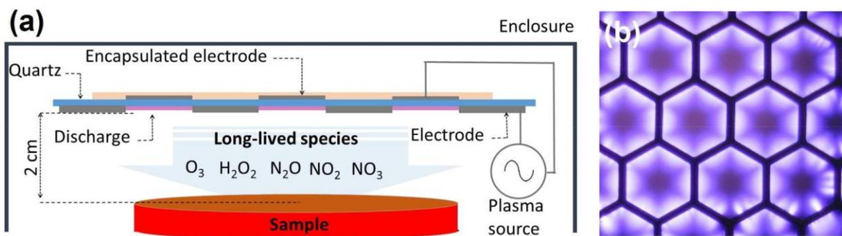
Figure 2. (a) Schematic showing surface DBD electrode and sample position, (b) Photograph showing plasma formed on hexagonal mesh electrode at a discharge power of  $0.67 \text{ W/cm}^2$ .
