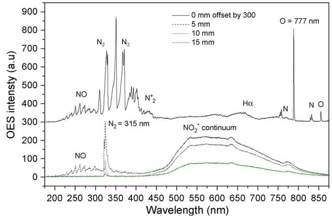
Fig. 1. Low-resolution OES (200–850 nm) of the discharge afterglow as a function of axial distance (0, 5, 10, and 15 mm). Drive frequency = 25 kHz, PCT = 100%, and air volume flow = 76.6 L/min.
