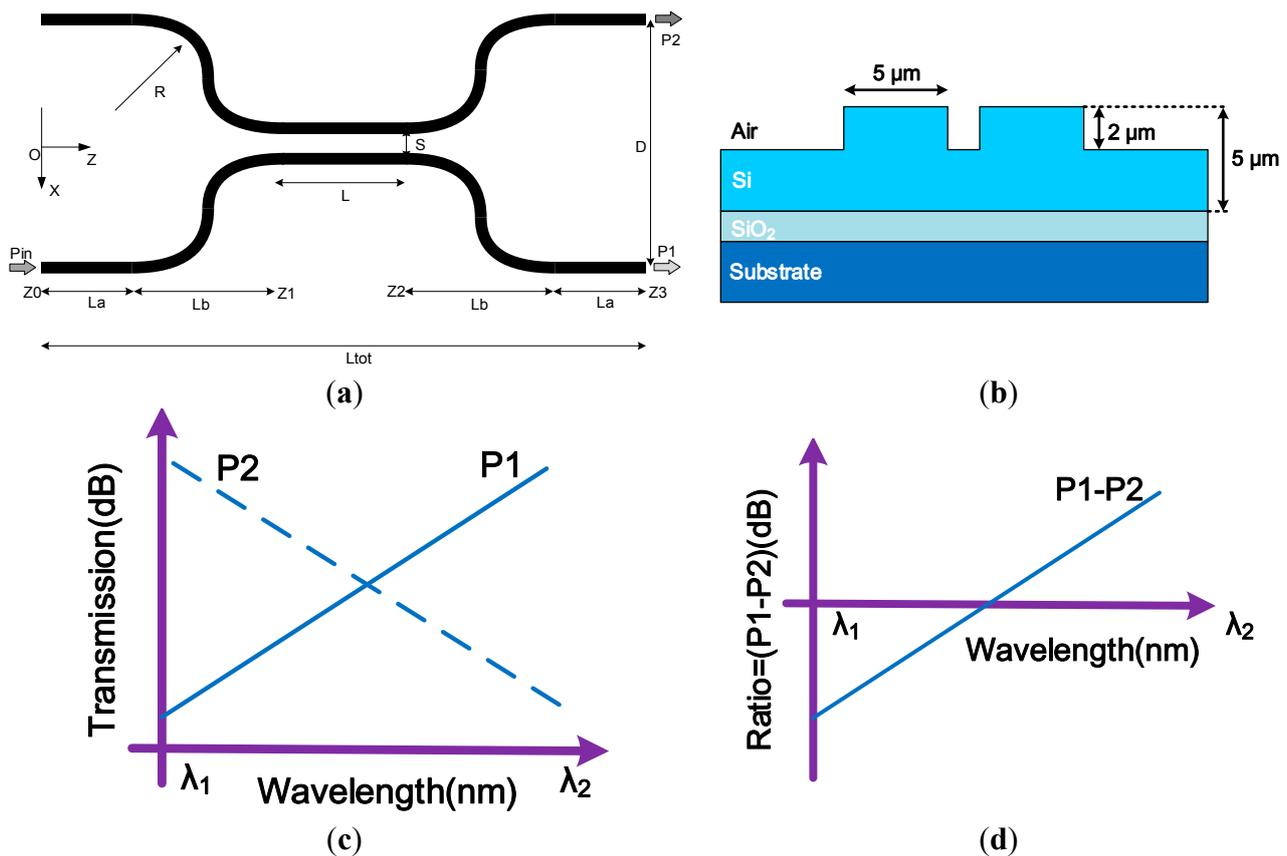
**Figure 1.** (a) Schematic structure of an integrated ratiometric wavelength monitoring based on a directional coupler consisting of an input region, a central region and an output region; (b) schematic cross section of SOI waveguide directional coupler; (c) desired spectral response; (d) output ratio of the two arms over the wavelength range.
