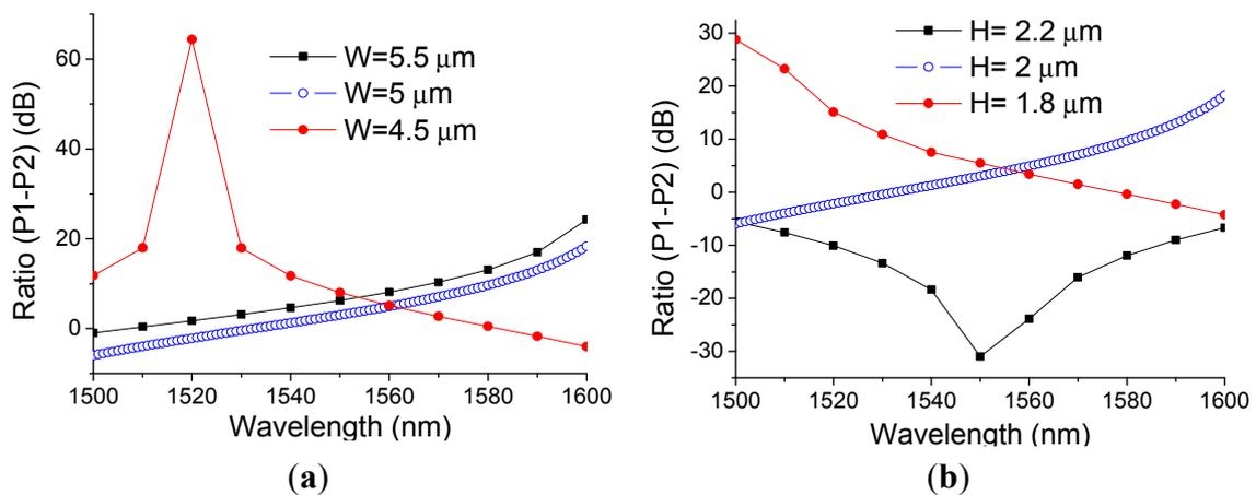
**Figure 8.** Ratio response of the designed structure with disturbed parameters: (a)  $W = 5 \pm 0.5 \mu\text{m}$ ; (b)  $H = 2 \pm 0.2 \mu\text{m}$ .
