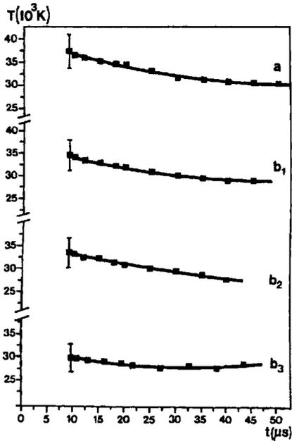
**Fig. 3.** Temporal evolution of the electron temperature ( $T$ ) at various discharge conditions:  $a$  ( $8 \mu\text{F}$ ,  $4.5 \text{ kV}$ ,  $\Phi = 5 \text{ mm}$ ,  $H = 6.2 \text{ cm}$ ),  $b_1$  ( $14 \mu\text{F}$ ,  $4.2 \text{ kV}$ ,  $\Phi = 25 \text{ mm}$ ,  $H = 14 \text{ cm}$ ),  $b_2$  ( $14 \mu\text{F}$ ,  $3.4 \text{ kV}$ ,  $\Phi = 25 \text{ mm}$ ,  $H = 14 \text{ cm}$ ),  $b_3$  ( $14 \mu\text{F}$ ,  $2.6 \text{ kV}$ ,  $\Phi = 25 \text{ mm}$ ,  $H = 14 \text{ cm}$ )
