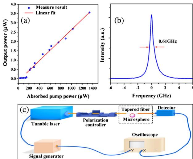
**Fig. 5.** (a) Microsphere laser output power as a function of estimated absorbed pump power at 1305.8 nm. The straight red line is a linear fit to the experimental data. (b) Oscilloscope trace of the Bi-doped microsphere laser recorded as the pump is scanned in frequency. (c) Schematic of the experimental setup for the linewidth measurement of Bi laser emission.
