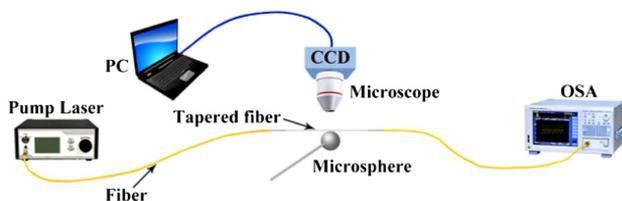
**Fig. 3.** Experimental setup for characterizing a Bi-doped microsphere laser. An 808 nm laser diode is used as the excitation source.
