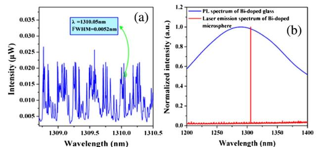
**Fig. 4.** (a) WGMs observed when light is coupled into doped microsphere via the fiber taper coupler. (b) Laser emission (red curve) from the Bi-doped microsphere when the absorbed pump power reaches 215 μW. As a reference, the fluorescence spectrum from the Bi-doped multi-component glass is also shown (blue curve).
