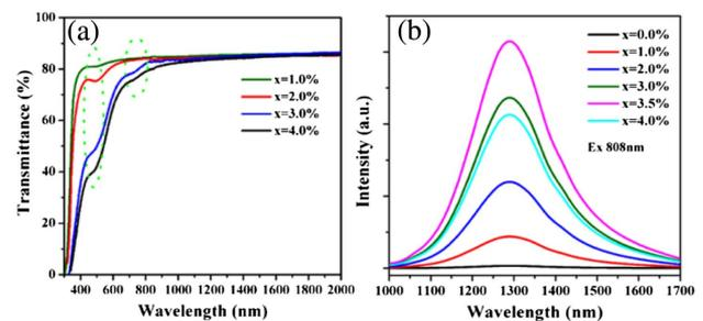
**Fig. 1.** (a) Transmission spectra of  $x\text{Bi}_2\text{O}_3$ -doped germanate glasses ( $x = 1.0, 2.0, 3.0,$  and  $4.0$ ). The different absorption bands around 500 and 800 nm over the transmission spectra are marked by two green dashed elliptical circles. (b) Photoluminescence spectra of  $x\text{Bi}_2\text{O}_3$ -doped germanate glasses under 808 nm excitation ( $x = 0.0, 1.0, 2.0, 3.0, 3.5,$  and  $4.0$ ).
