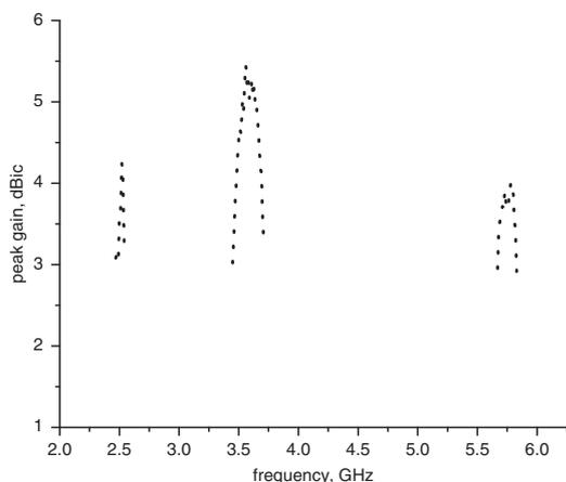
**Fig. 6** Measured peak gain for proposed antenna
