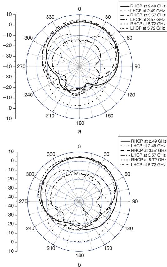
**Fig. 5** Measured radiation patterns
