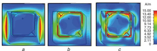
Fig. 2 Surface current distributions for three frequency bands
