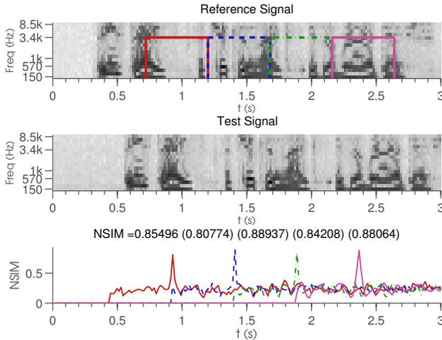
**Fig. 1.** Speech Signals with sample patches. The bottom plot shows the NSIM similarity score for each patch from the reference compared frame by frame across the test signal. The NSIM score is the mean of the individual patch scores given in parenthesis.
