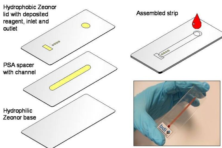
**Figure 1.** Schematic and photograph of the microfluidic anti-FXa assay device. Strips were assembled from a hydrophobic Zeonor lid containing an inlet and outlet. The single straight channel was cut from PSA which seals the lid and base layers. The base layer was hydrophilic Zeonor to allow for capillary fill of the strip. Fluorogenic FXa substrate was deposited onto the hydrophobic lid prior to assembly.
