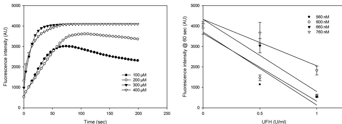
**Figure 3.** (a) Typical fluorescence profiles of the anti-Xa assay at a fixed concentration of FXa and varying concentrations of Pefafleur™ FXa; (b) Fluorescence responses at 60 s for a range of FXa concentrations and a fixed concentration of Pefafleur™ FXa at 0, 0.5, and 1 U/ml UFH (n=3).
