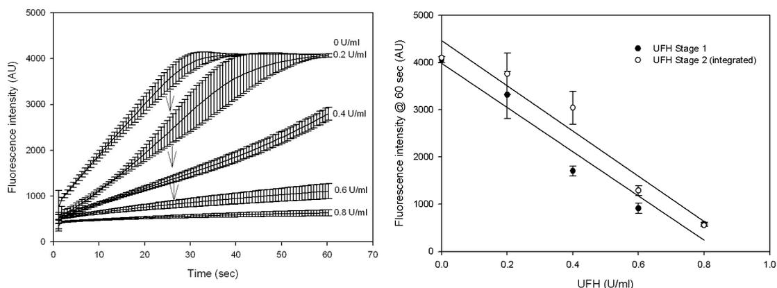
**Figure 4.** (a) Fluorescence response profiles of human plasmas in the anti-Xa assay device supplemented with concentrations of UFH from 0 – 0.8 U/ml (n=3); (b) Dose response curve of human plasma spiked with UFH from 0 – 0.8 U/ml in stage 1 and stage 2 (fully integrated) of the anti-Xa device (n=3).
