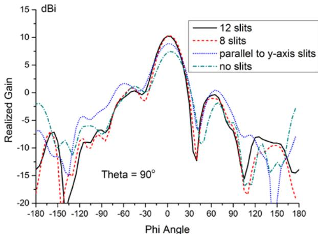
Fig. 7 Parametric study on ground plane slits
