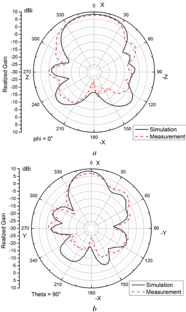
**Fig. 10** Simulated and measured realised gain at 28 GHz
