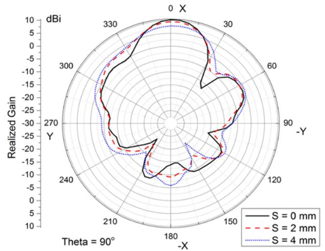
Fig. 8 Parametric study on slit position  $S$
