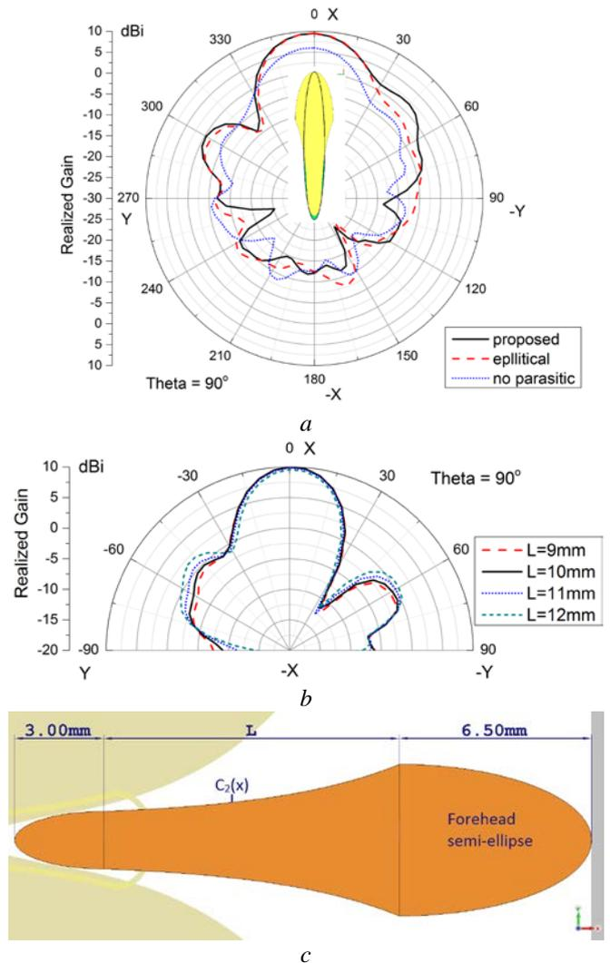
Fig. 5. Parasitic element study
