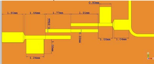
Fig. 3. Detailed bandpass filter layout
