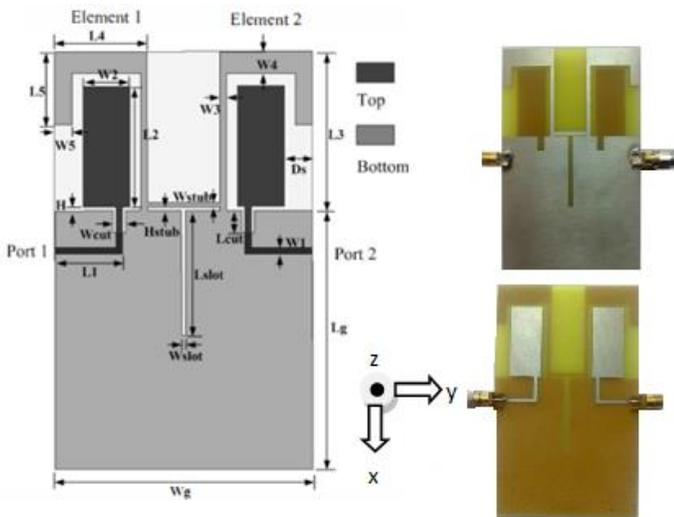
Fig. 3. Geometry of final design and prototype
