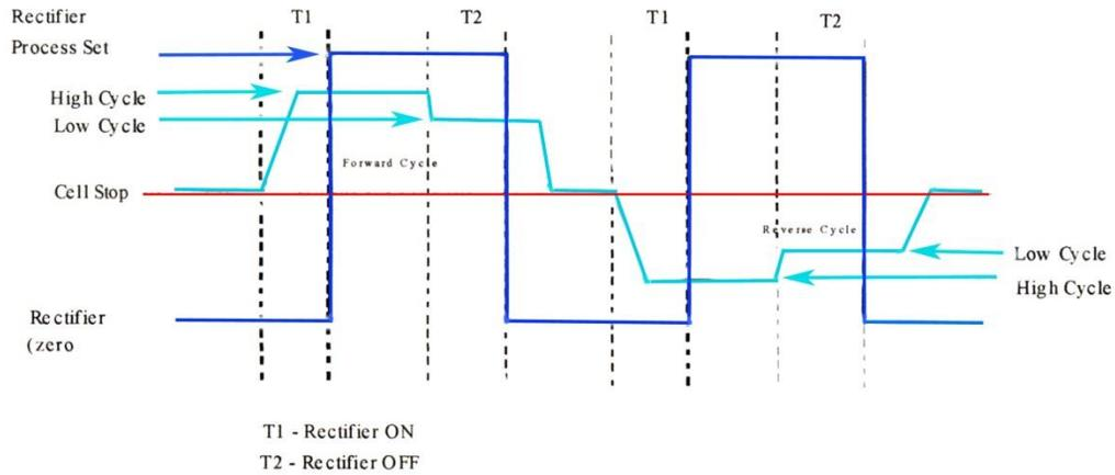
**Figure 4 RFT Cell Rotation and Rectifier current relationship**
