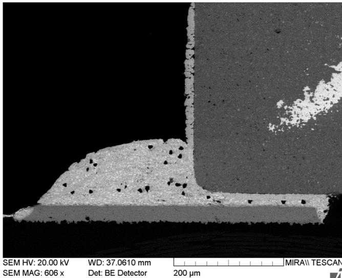
**Figure 8 SEM image with back scatter detector of AgPt solder fillet height in cross section showing <40% fillet height. This image the solder pad loaded with solder, the dark grey ceramic chip and the thin porous layer of the Ag/Pt termination is visibly leaching into the solder paste.**
