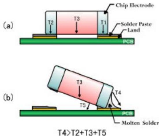
**Figure 2 Forces causing tombstoned device (courtesy of A. Takaki, Senju Advanced soldering Technology)<sup>5</sup>**
