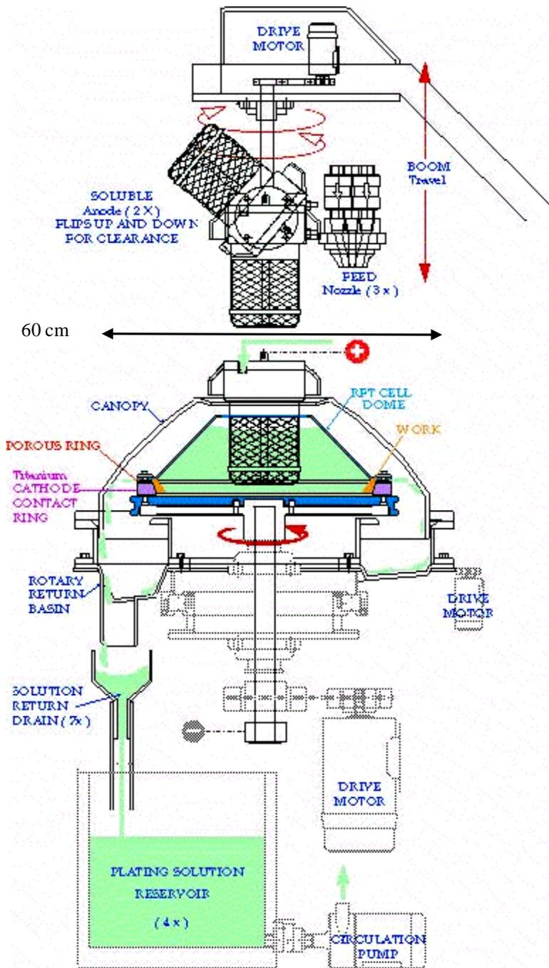
**Figure 3 Schematic of Rotary Flow Thru' Plater**
