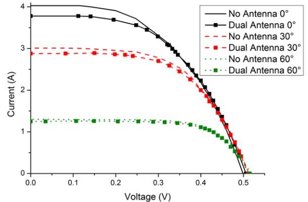
Fig. 6. Measured solar output at various incident angles
