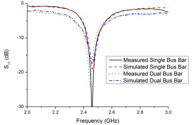
Fig. 3. Measured and simulated antenna  $S_{11}$  results
