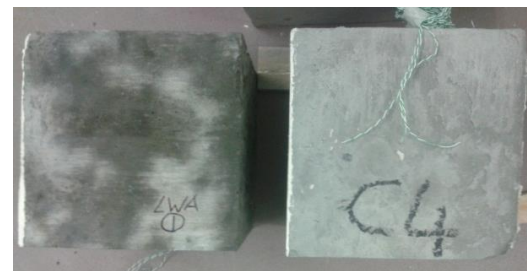
Figure 5. Leakage of PCM from the lightweight aggregate
