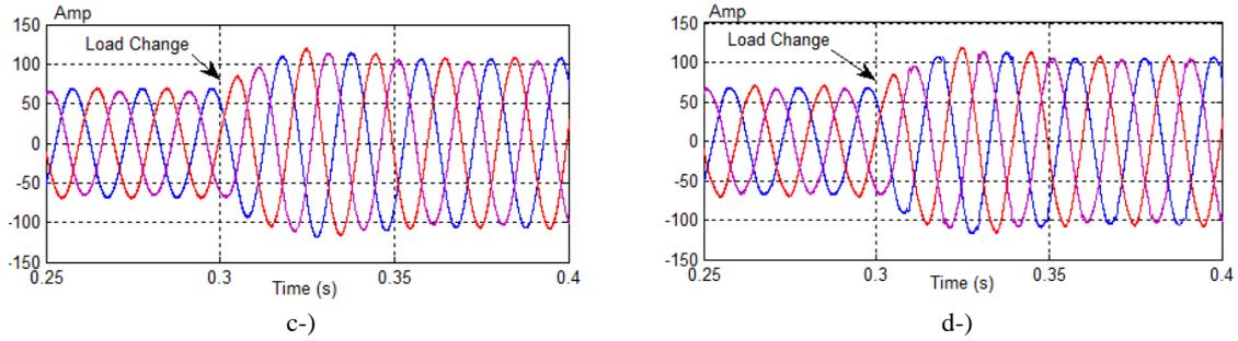
Fig. 3. Compensation of the grid current harmonics by using conventional  $dq$  method: a-) under ideal voltage, b-) under non-ideal voltage, and by using conventional  $pq$  method: c-) under ideal voltage, d-) under non-ideal voltage,
