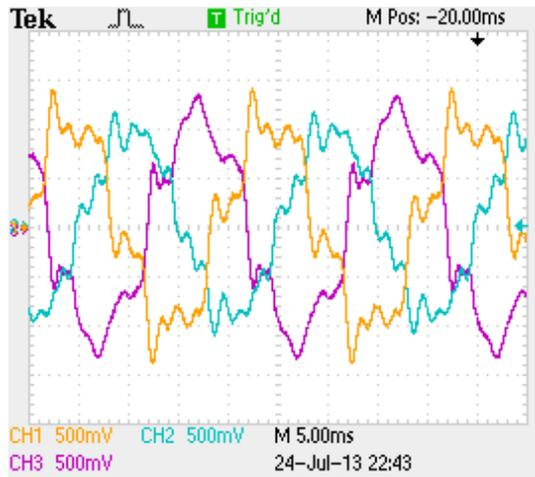
Fig. 8. Three phase non-linear load currents (scale: 47 A/div.)
