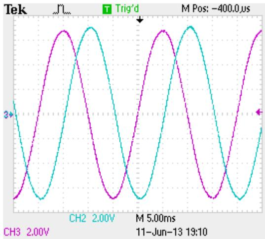
Fig. 7 (c). Output signal of the STF ( $\bar{u}_\alpha, \bar{u}_\beta$ )
