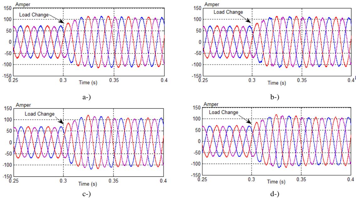
Fig. 4. Compensation of the grid current harmonics a-) by using STF based *pq* theory under ideal voltage, b-) by using STF based *pq* theory under ideal voltage, c-) by using proposed method under ideal voltage, d-) by using proposed method under non-ideal voltage
