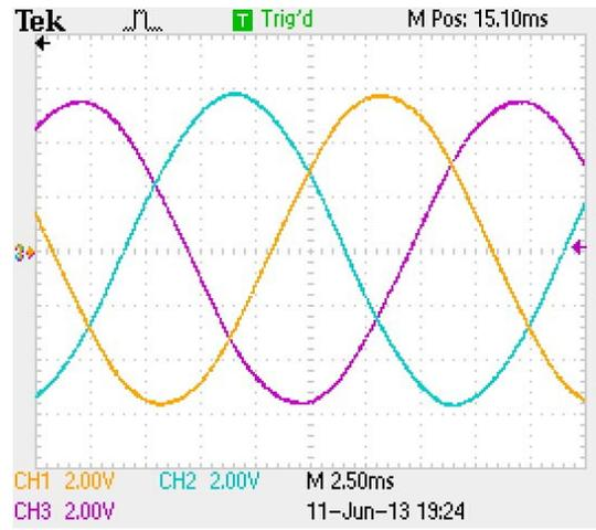
Fig. 7 (d). The obtained three phase balanced and un-distorted
