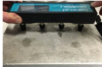
Figure 6 Resipod used for Resistivity Measurements
