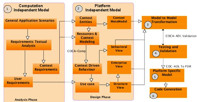
**Figure 1. Context-oriented Component-based Application Model-Driven Architecture (COCA-MDA)**
