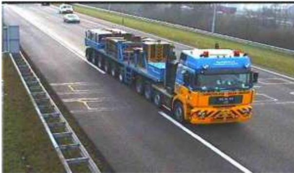
(c) Crane ballast truck (109 tonnes, 10 axles).
