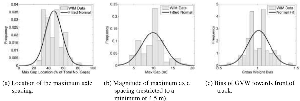
Figure 6. Histograms of low loader characteristics at Czech Republic site with fitted normal distributions.
