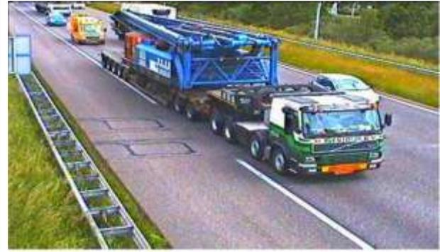
(b) Low loader (127 tonnes, 11 axles).
