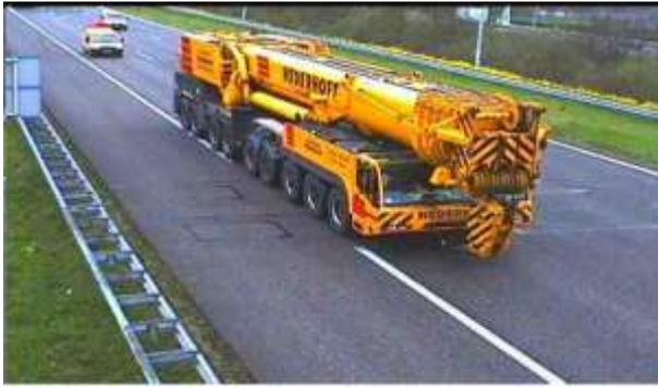
(a) Mobile crane (109 tonnes, 9 axles).
