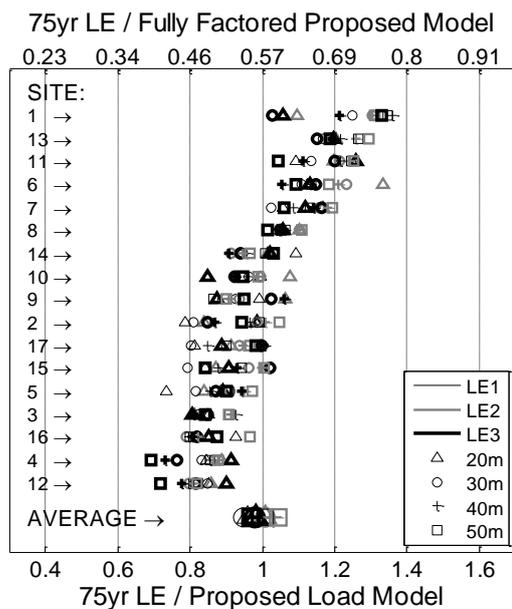
Figure 7. Single-lane characteristic load effects, normalized with respect to proposed variable UDL load model (mean of site standard deviations is 0.064).
