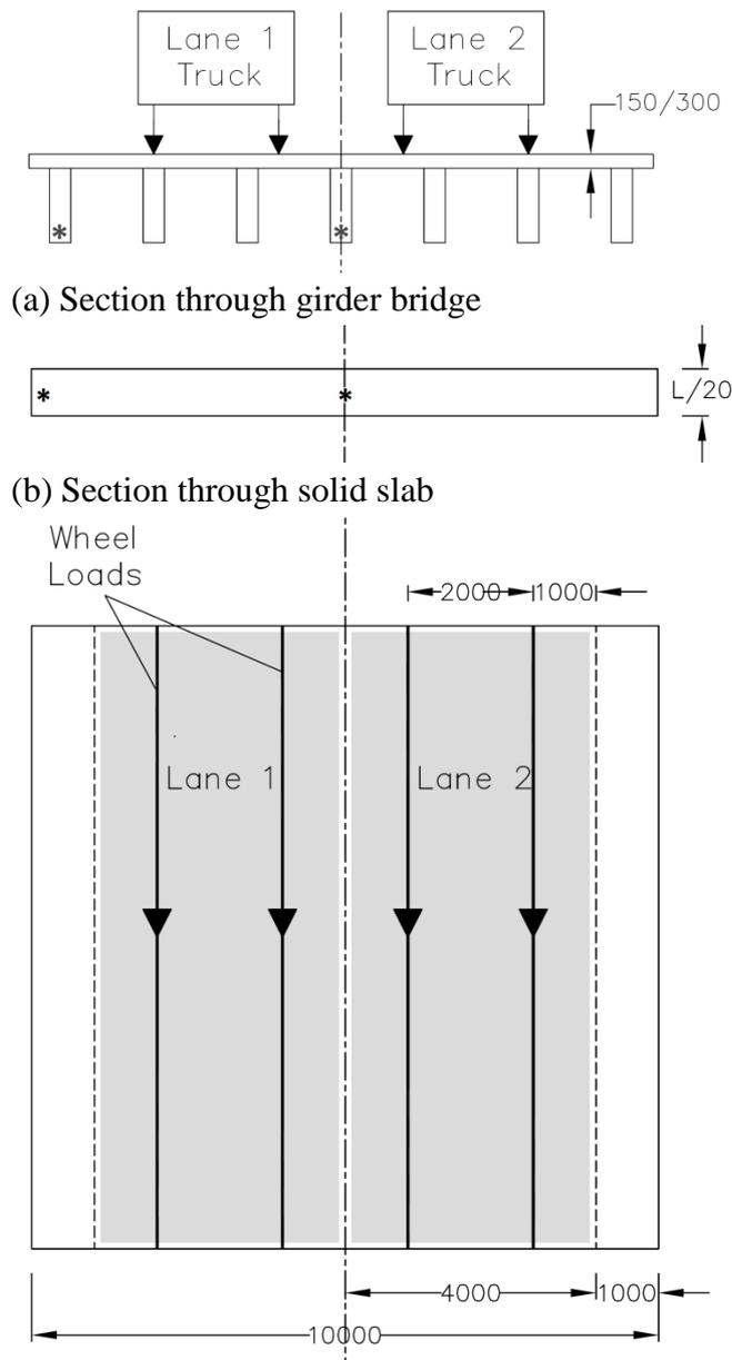
Figure 4. Bridges used in the two-lane same-direction analysis (\* = locations where load effects are examined).
