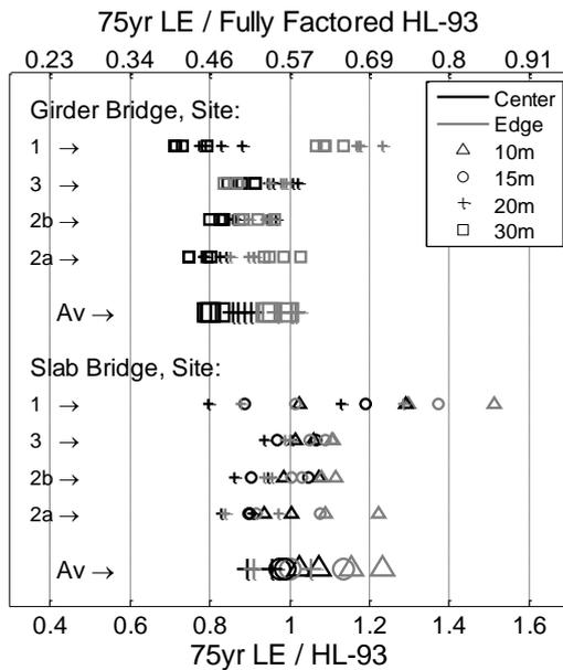
Figure 8. Two-lane same-direction characteristic load effects, normalized with respect to HL-93.
