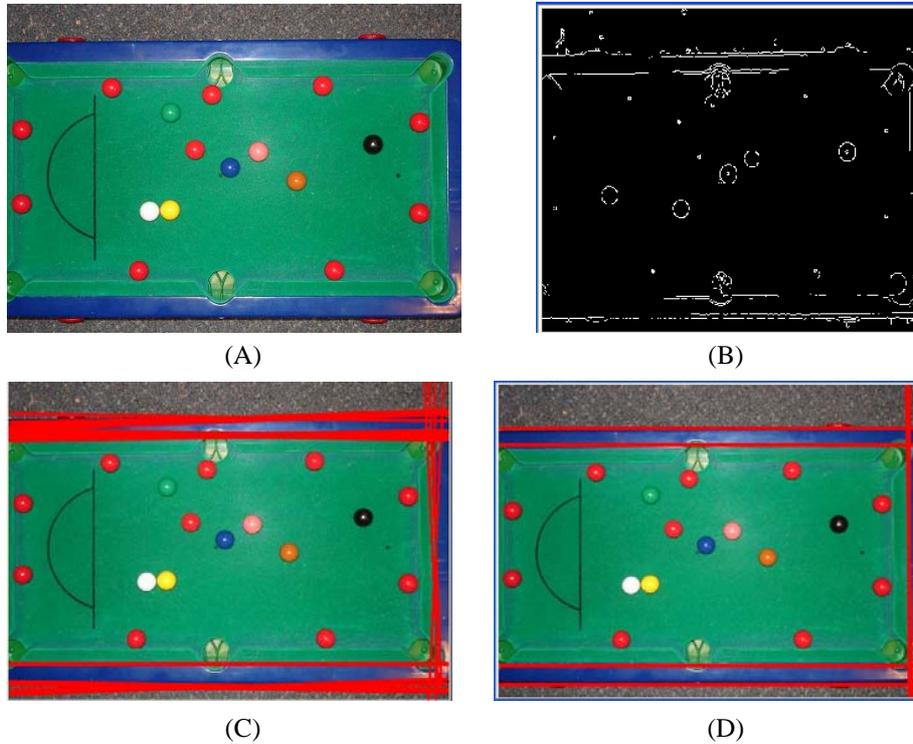
**Fig. 1.** (A) The original image, (B) the edge detection result, (C) the results of a Hough transform super-imposed on the original image and (D) the final extracted table boundary super-imposed on the original image.
