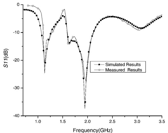
**Figure 9** Comparison of the simulated and measured  $S_{11}$  for Antenna B
