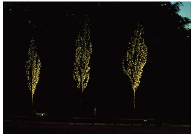
Figure 6: Narrow beam uplighters focus light on trees and limit upward glare.
