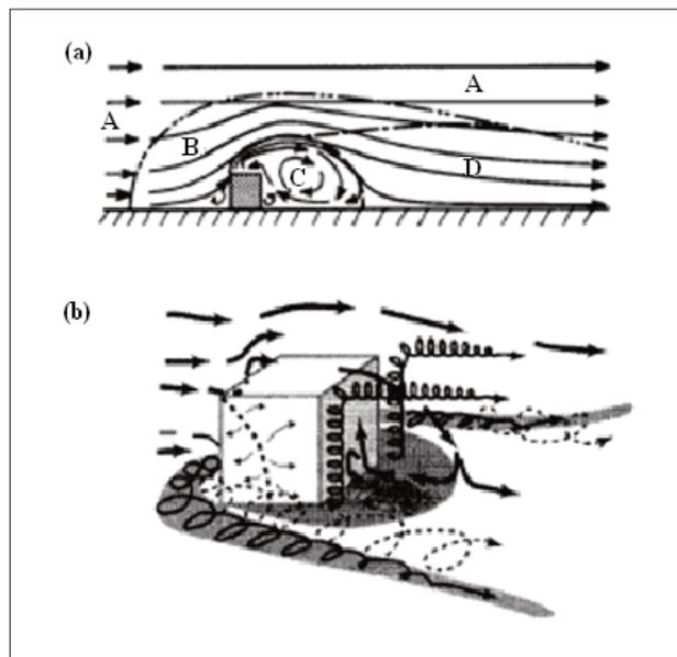
Figure 3: Two-dimensional flow around a building with flow normal to the upwind face (a) stream lines and flow zones; A – undisturbed; B – displacement; C – cavity; D – wake; and (b) flow, and vortex structures (Figure 3 courtesy Oke, 2006)
