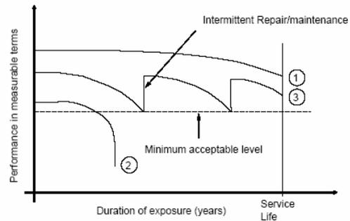
**Fig. 2** Service life performance of reinforced concrete structures
