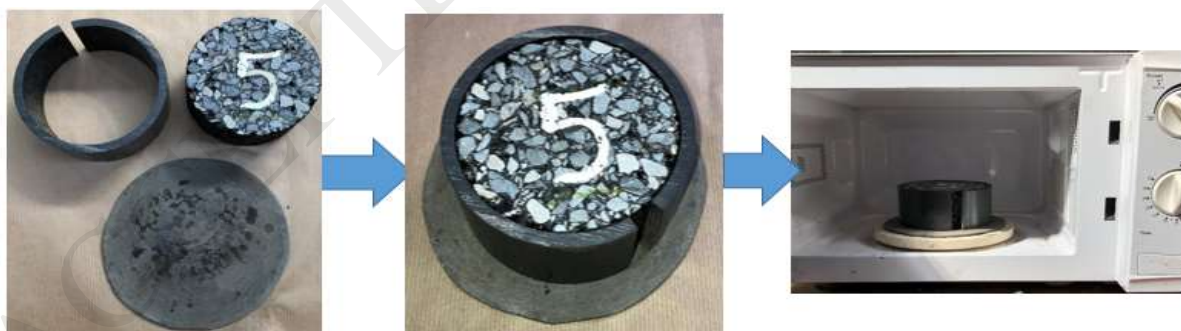
Figure 3. Microwave healing test system set up.
