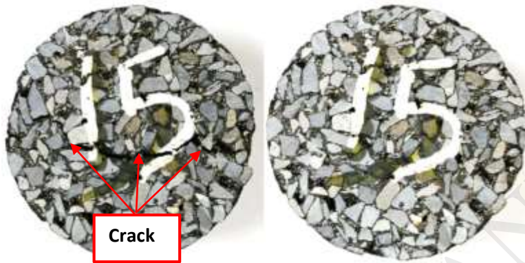
Figure 13. PFC specimen #15 with 15% steel fibre: Left: before healing and Right: after healing with fully repaired crack.
