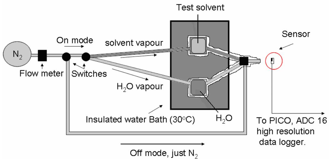
Figure 2. Bubbler apparatus schematic, the Dreschel flasks typically held a volume of  $40 \text{ cm}^3$ .
