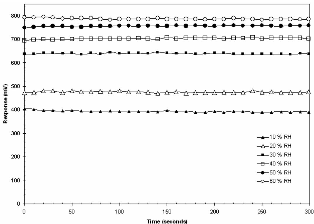
Figure 10. Graphical representation of sensor's response to increasing % RH over time at a constant temperature of 23.1°C.
