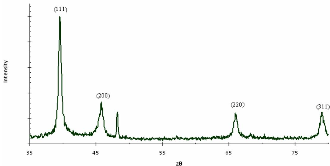
Figure 6. XRD pattern recorded from a drop-coated film of Ag/polymer nanocomposite on glass substrate.
