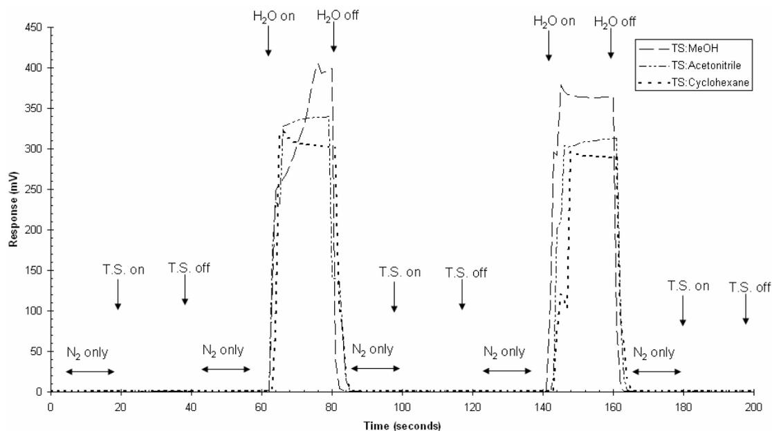
Figure 8. Sensor's response to exposure to various solvent vapours, summarised in Table 1. Exposure was conducted using the bubbler apparatus, where the streams passing over the sensing membrane were 'switched' from the reference gas to either the test solvent (T.S.) or water vapour as indicated.
