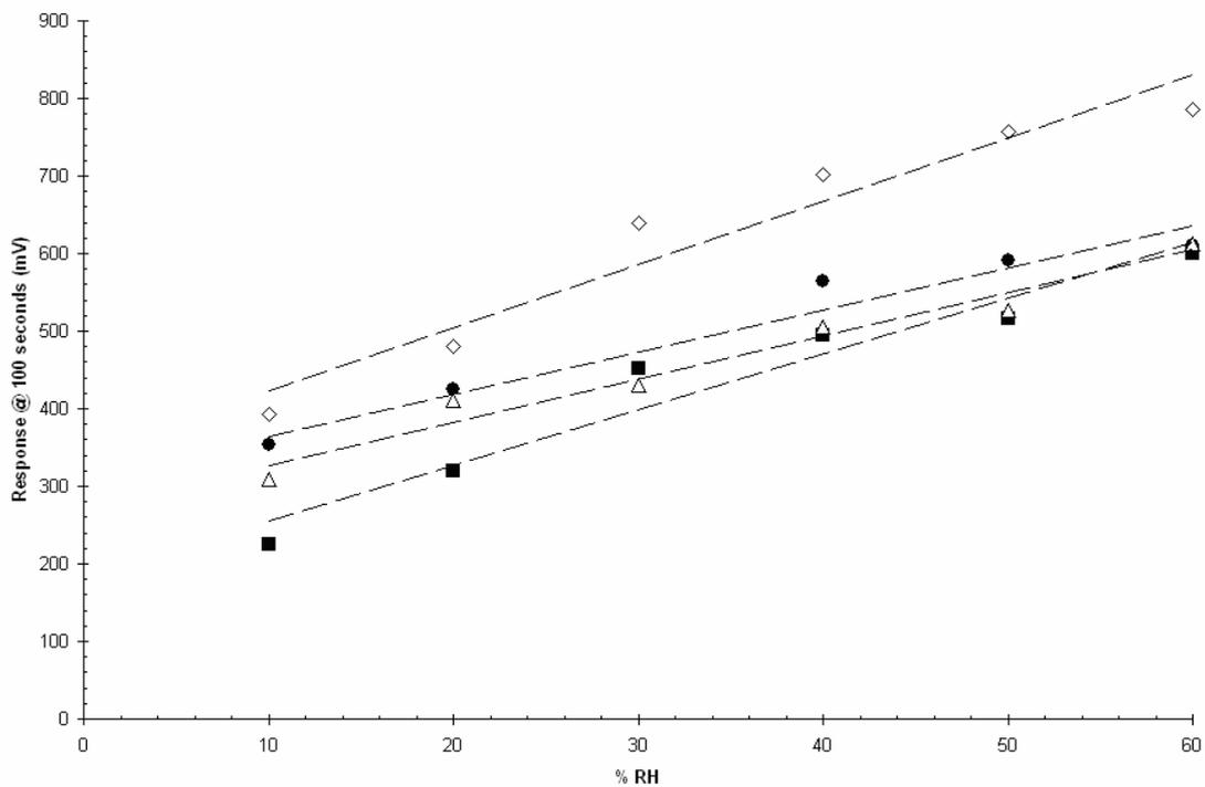
Figure 12. Responses of four different sensors prepared separately. The slopes for the lines are 5.4, 5.5, 7.2 and 8.2 (mV/%RH).
