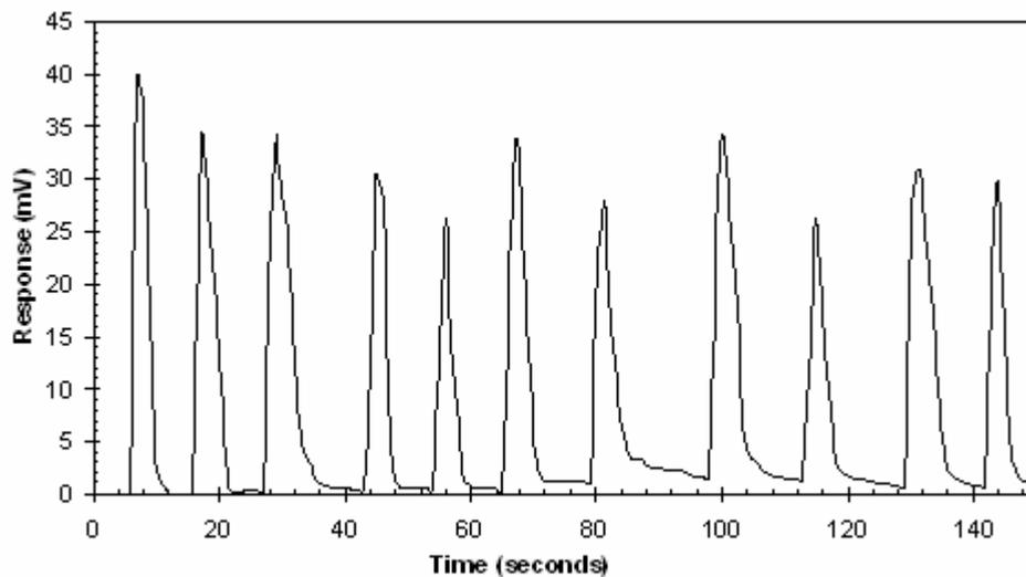
Figure 7. Representative plot of sensor's response to a change in environment. The sensing membrane was repeatedly exposed to water vapour at regular time intervals.
