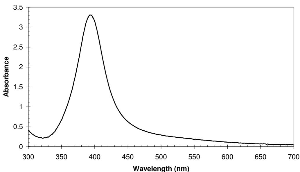
Figure 3. UV-Vis spectrum of stable aqueous colloidal Ag polymer mixture, with  $\lambda$  max of 391 nm.  $[\text{Ag}^+] = 1\text{M}$  ( $0.5\text{cm}^3$ ),  $[\text{PVA}] = 1\%$  wt/wt ( $0.66\text{ cm}^3$ ),  $[\text{NaBH}_4] = 0.1\text{M}$  ( $6\text{cm}^3$ ) diluted to  $10\text{cm}^3$  and maintained at a low temperature.
