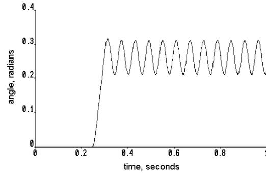
Fig. 10. Oscillations due to setting  $k_i$  just above its threshold value.
