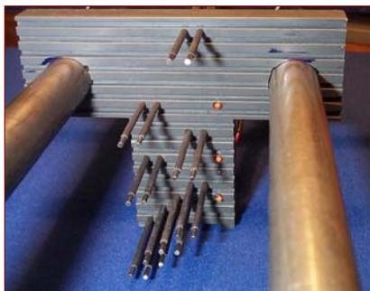
**Figure 1.** *The multi-electrode array*
