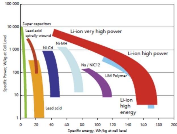
Figure 4: Specific power and energy by battery technology [2]
