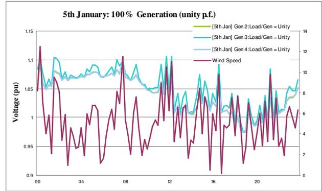
Figure 5: Voltage variation with respect to wind speed for the 5<sup>th</sup> January
