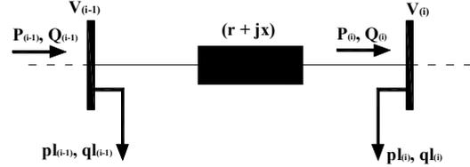
Fig 2. Radial Feeder
