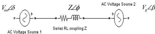
Figure 1: Power flow between two AC Sources
