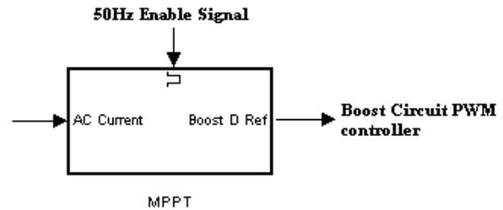
Figure 4: MPPT Controller for the novel approach
