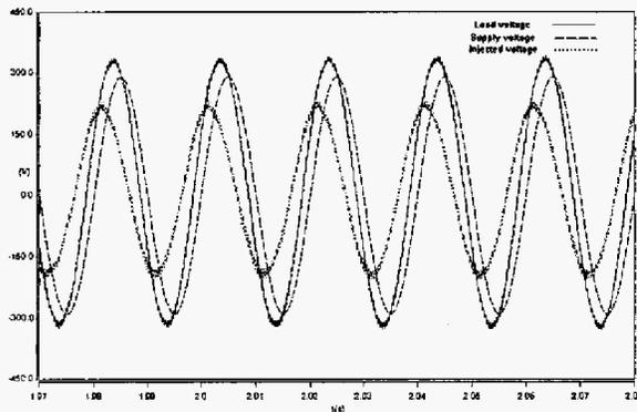
Fig. 7 Load, Supply and Injected Voltage at SC
