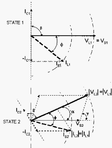
Fig. 3 Phasor diagram of UPQC for States 1 and 2
