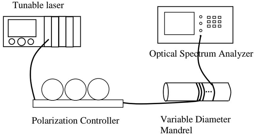
Fig. 5. Experimental setup for measuring polarization dependent loss.
