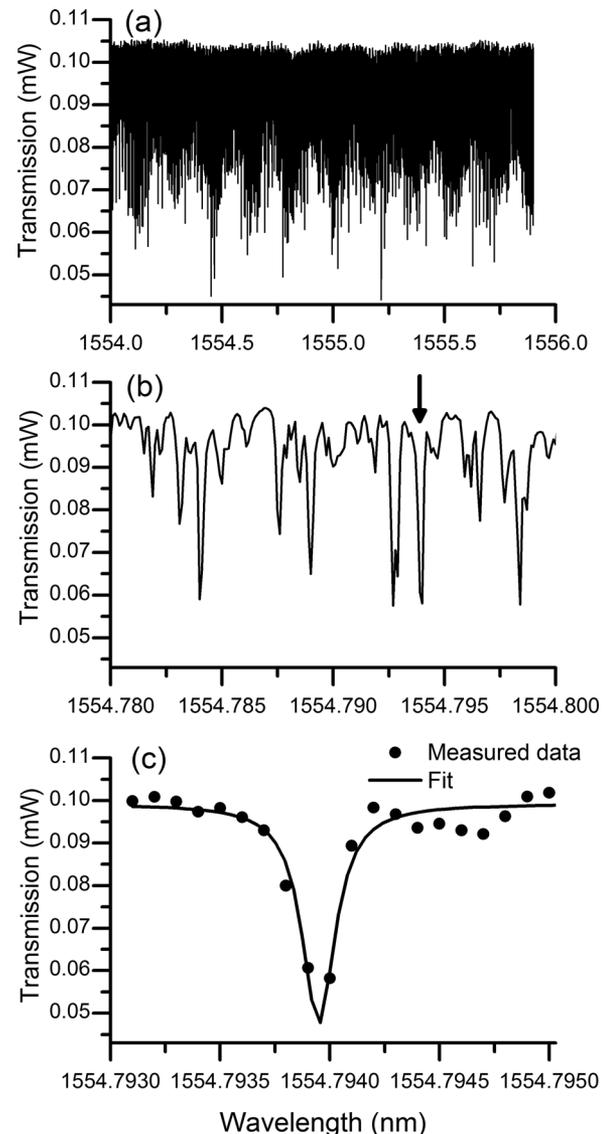
FIG. 4. (a) Experimental resonance spectra for wavelengths between 1554 and 1555 nm for the microsphere with diameter 109  $\mu\text{m}$  (b) Close-up spectrum in the region 1554.78–1554.80 nm clearly showing the high- $Q$  resonances and (c) a Lorentzian fit to one of the measured tuning-resolution limited resonance dips used to accurately determine the bandwidth.
