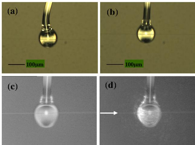
FIG. 3. (Color online) Microscope images of lead-silicate microspheres with diameters (a) 103  $\mu\text{m}$  and (b) 109  $\mu\text{m}$  showing their fiber stems and the tapered coupling fibers. (c) and (d) show the infrared images of the microsphere when the input laser light is turned off and on, respectively.
